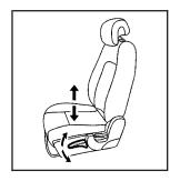
If your vehicle has a manual driver seat height adjuster, it is located on the outboard side of the seat near the front of the seat cushion.
